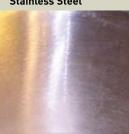
\$85-100/sq. ft. A combination of steel, chromium and nickel. Its production requires large amounts of energy. Chromium, a toxic heavy metal, is bound in stainless steel during manufacturing so the finished product is nontoxic (although there still is an issue with pollution caused by its production).
